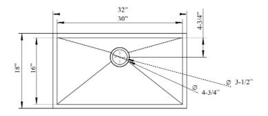
Dimensions of fixture are nominal and may vary within the range of tolerances established by ANSI Standard A112.19.2. Dimensions and specifications subject to change without notice.
